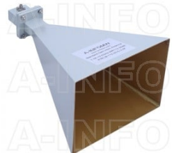
LB-112-20-C-3.5F Standard Gain Horn Antenna 7.05-10GHz 20dB Gain 3.5mm Female
